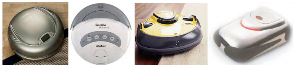
Figure 5. Current consumer robotic vacuums: Electrolux Trilobite, iRobot Roomba Discovery, Kärcher Robocleaner, and Zucchetti Orazio.
